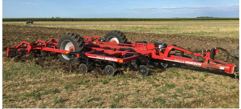
A Horsch high speed tillage disc working up perennial forage stand in the fall after being sprayed out.
