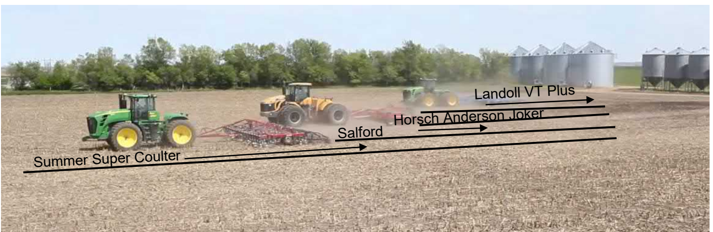
Above is a clip from a youtube video called Horsch Anderson Joker versus Salford RTS, Summers Supercoulter & Landoll VT Plus that shows the different level of disturbance from vertical & high speed tillage implements. The vertical tillage choices include Summer Super Coulter (closest to the bottom pass that has already gone by) & Salford RTS (second from the bottom). The high speed tillage include a pass using the Horsch Anderson Joker implement (third pass from the bottom; notice the black soil behind from the more aggressive disturbance and incorporation of straw). The final pass is with a Landoll VT plus (closest to the top).
